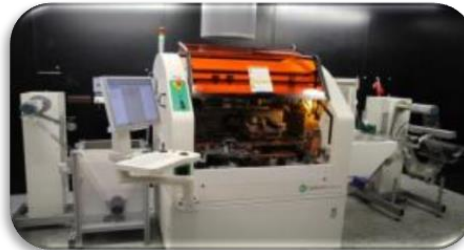
Roll-to-roll assembly and bonding line
