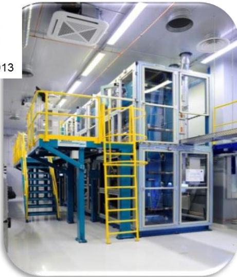
MAXI – In-air roll-to-roll pilot line
